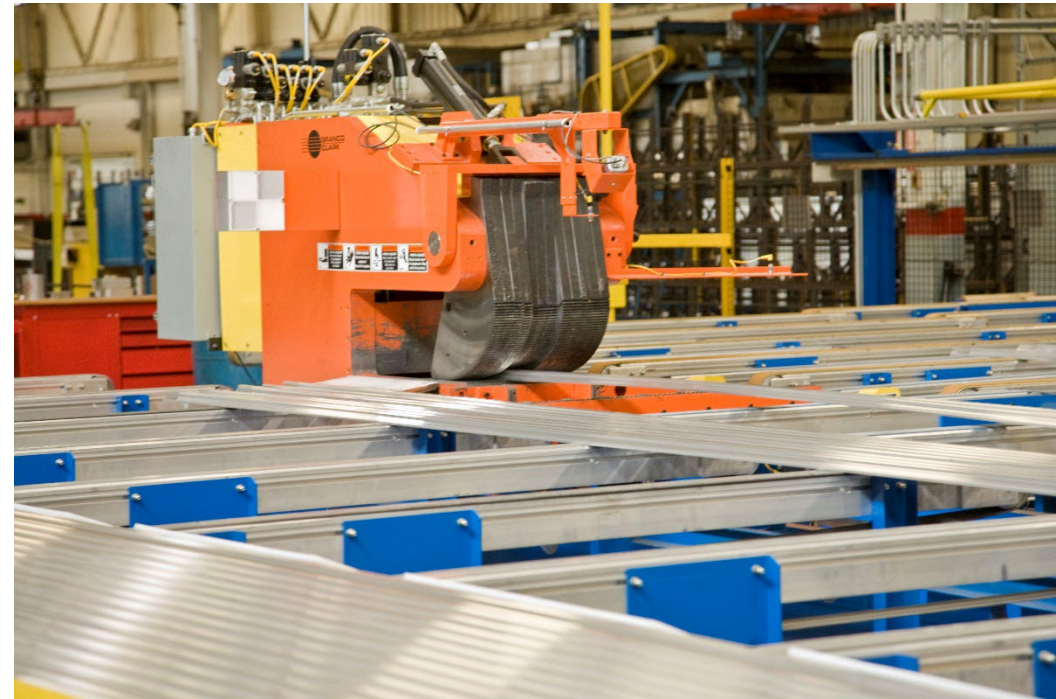
A stretcher can be used to help achieve desired straightness requirements.
